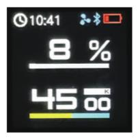
3. Short press the brightness adjustment knob or color temperature adjustment knob to quickly adjust the gear: the brightness can be quickly adjusted to 0%, 25%, 50%, 75%, and 100%; The color temperature can be quickly adjusted to 2700K, 3500K, 4500K, 5500K, 6500K.
