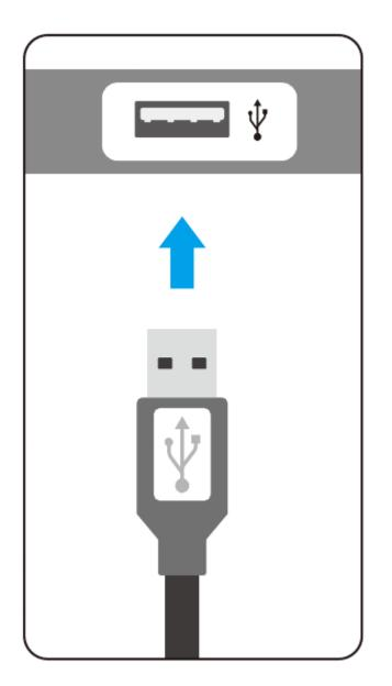
Plug the USB connector into the mobile device via an OTG cable.
