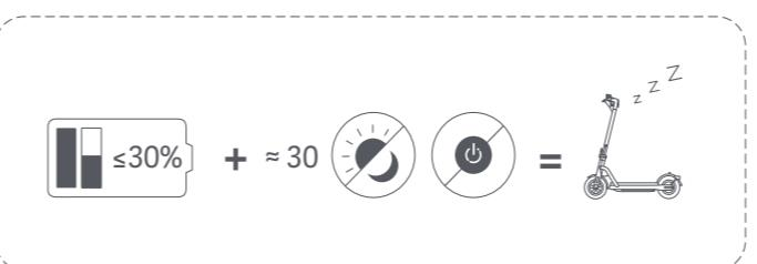
EN When the scooter is turned off for about a month with the battery level of the scooter being lower than 30%, the scooter will enter sleep mode. In this case, the scooter cannot be turned on. To exit the sleep mode, charge the scooter for about three seconds to activate the battery.
