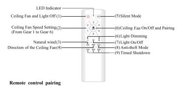
Ceiling Fan On/Off and Pairing: key (0) is the ceiling fan on/off and pairing key. When the ceiling fan is on, press this key to turn off the ceiling fan. Within 15 seconds after power -on, long press this key for about 2 seconds to pair the remote control, and the buzzer will beep three times to indicate that the pairing is successful.
