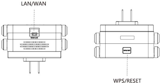
Tip:Hold down the RESET key for 5 seconds to reset the device
