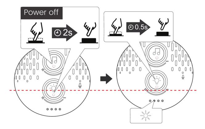
When the Bluetooth speaker and lights are turned off, press and release the lamp button for 0.5 seconds to trigger the fast charge output and battery indicator.
