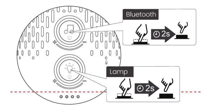
**Lamp:** Long press the lamp button for 2S to turn on/off the lamp.
