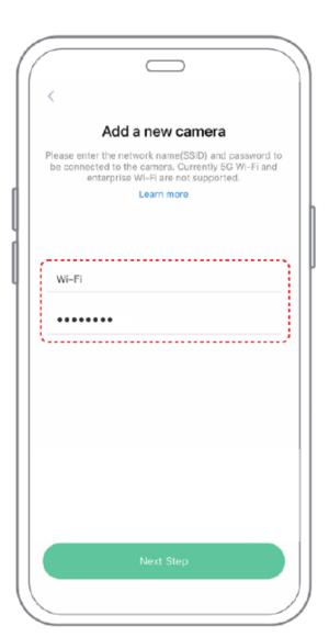
2) To ensure a longer distance connection, the camera only supports the 2.4Ghz Wi-Fi with stronger wall penetration capability and does not support Wi-Fi for enterprise level authentication currently. Please ensure that the entered Wi-Fi meets the requirements. After completion, click "Continue" to generate the QR code for pairing the camera.
