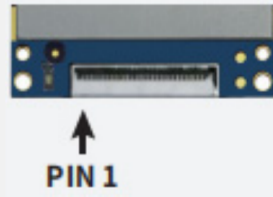
FPC connector (30Pin , Space between PINs 0.5mm)
