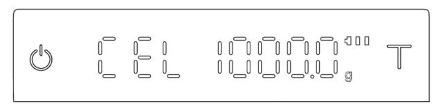
3. Once you have selected the maximum capacity you wish to use, press the power button once and "c-2ero" will flash after the calibration mode has been enabled and then the display will show "PUT 100g".
